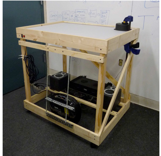
Figure 2: Second-generation multi-touch table, incorporating FTIR sensing, haptic feedback, and a simplified two-channel audio display used during development. Note the transducer coupled directly to the surface of the table at the top right.
